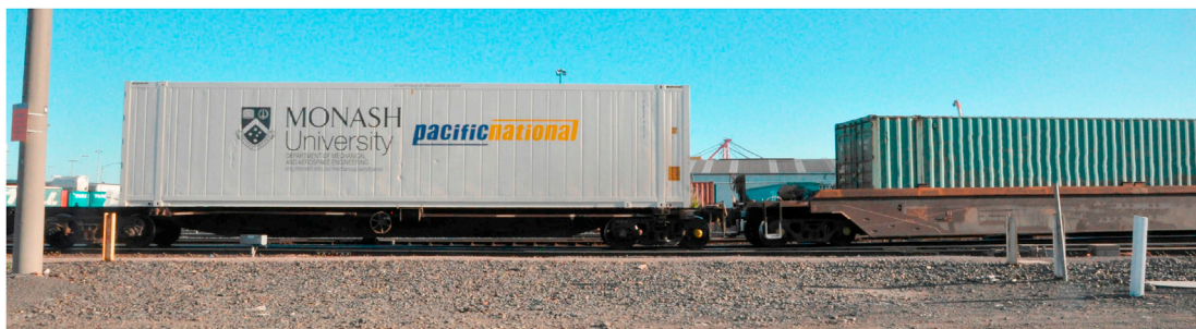
Fig. 1. Instrumented 48 ft refrigeration shipping container (white, front) on board an operational freight train with significantly flatter external ridges than conventional containers (green, back). (For interpretation of the references to colour in this figure legend, the reader is referred to the Web version of this article.)
