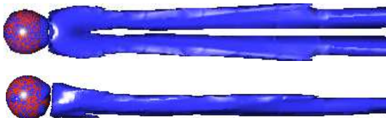
(b) Numerical simulations showing the steady wake from above and from the side.
