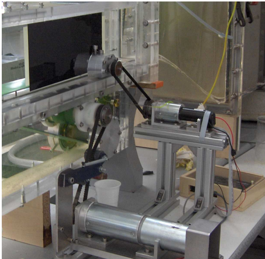
FIGURE 3.4: View from the back of the test section, showing the two motors that are used to drive the moving floor and the cylinder/sphere assembly.
