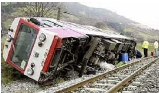
Figure 1 Cross-wind related accident in Austria, 2002
