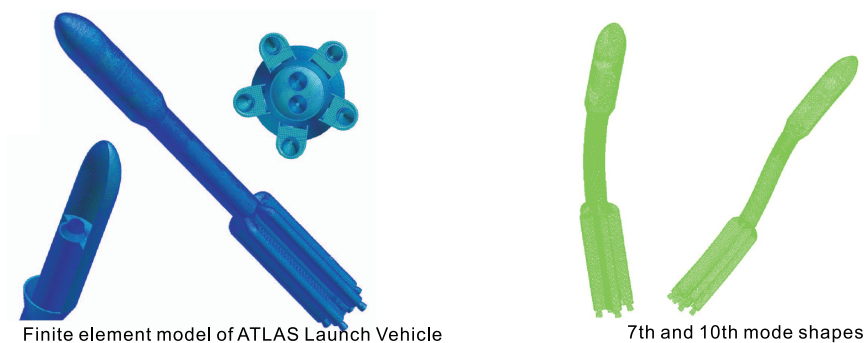
Figure 4: Finite element model and natural mode shapes of ATLAS V500 launch vehicle
