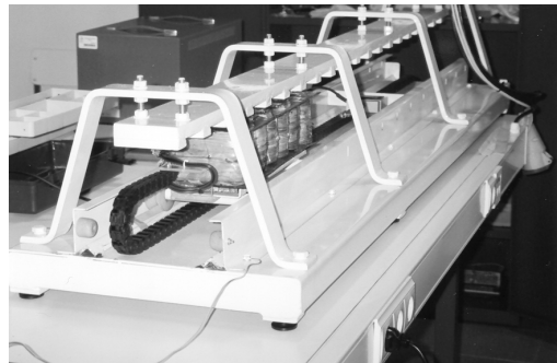
Figure 1 LSRA prototype mounted on a test bench
