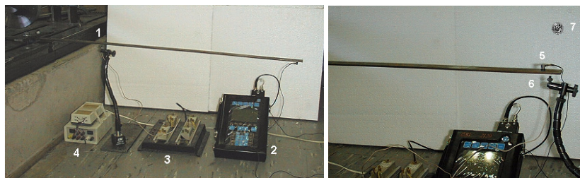
Figure 2. Experimental set up: 1 cantilever beam (had length L=1.15 m, width A=0.02 5m, and thickness E_s=0.005 m. The mechanical characteristics are, E=2.1 \cdot 10^5 MPa, density \rho=7850 kg/m 3 , and \sigma_0=340 MPa)., 2 analyzer, 3 amplifier, 4 source power, 5 accelerometer, 6 displacement sensor, 7 rigid ball.
