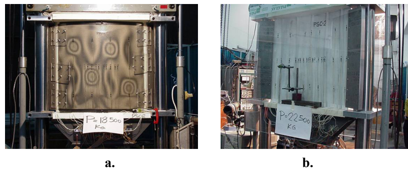
Fig.5 Panel PSC-2 at various postbuckling axial loads: a. at 180 kN (front), b. at 225 kN (back).
