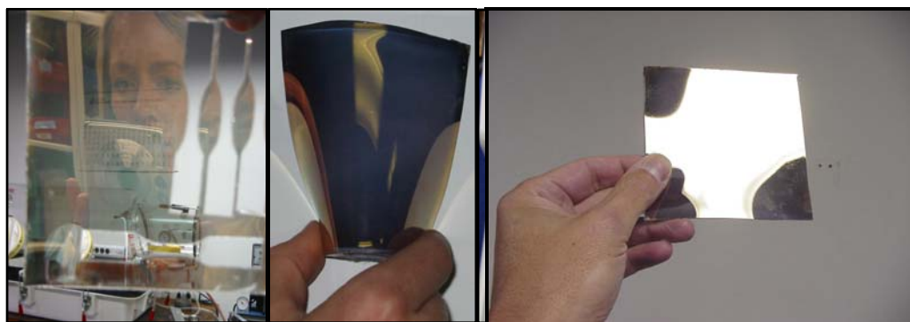
Figure 6. Metal Rubber Materials Formed by ESA Processing.
