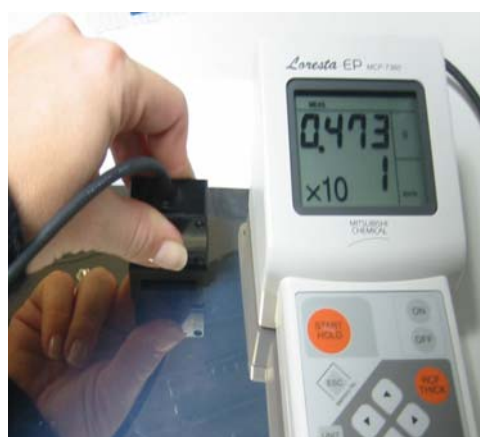
Figure 7. Metal Rubber Displays High Electrical Conductivity and Low Modulus.
