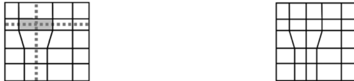
(a) Initial mesh and STC chords of selected element (b) Improved mesh
