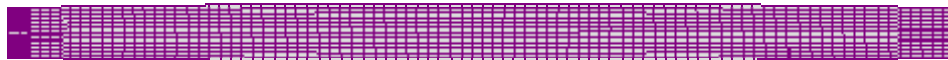
Figure 9: Refined mesh with mesh quality improvement: Max. aspect ratio 2.8 and average aspect ratio 2.4
