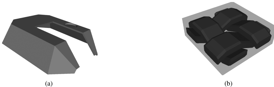
Figure 3: Multiscale model used in residual stress computations. a) Micro-scale unit cell model of woven fabric and resin. b) Snapshot of macro-scale composite part model.
