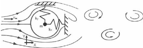
Figure 10: Scheme of the 2-DOF whirl resonance problem
