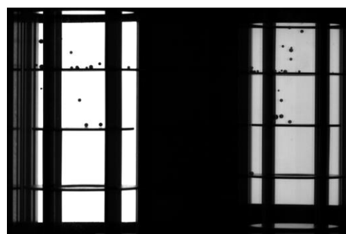
Figure 3 Example of drops visualization within the column (left) and 45° view on the mirror (right)
