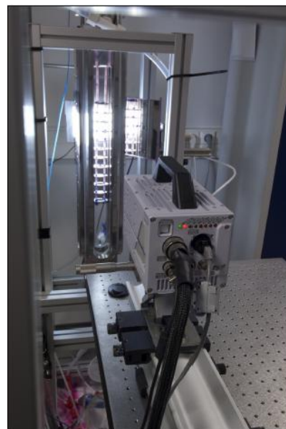
Figure 2: Experimental set-up for drop trajectory measurements
