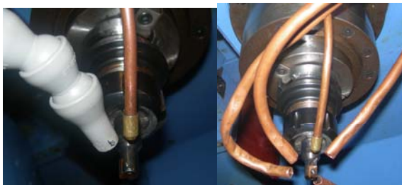
(a) VT+MQL (b) Four cooling nozzle+MQL Fig. 4 Cooling Parameters
