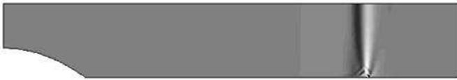
Fig. 7 Perturbation contours of vertical vorticity displaying strong growth around the source radius for Re = 4639 , k = 13 . Greyscale contours are used where light and dark shadings denote positive and negative values respectively.
