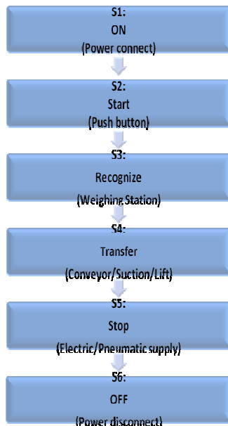
Fig. 2: Process Instructional Guide with Component Specification
