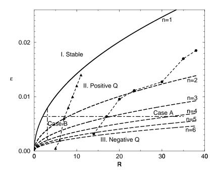
Figure 1. Stability diagram for Eqs.(1),(2) as presented in the  $\varepsilon - R$  plane. The curves n = 1 to n = 6 given by Eqs.(18),(19) show the instability thresholds for the n-th mode, thus n = 1 is the instability threshold of the system. The horizontal and vertical dot-dashed lines indicate the parameter values investigated here in the framework of cases A and B, respectively. The dashed curve marked with black circles displays the border line below which the value of Q becomes negative.
