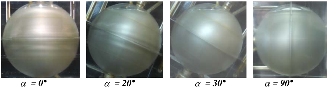
Figure 9: Effect of the inclination \alpha on the vortex of Taylor Ta=45, \Gamma= 18 (Relaminarization \alpha = \alpha_c = 30^\circ )
