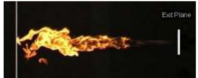
Figure 3: Example of instantaneous flame length measurement performed by software using frame-by-frame approach.
