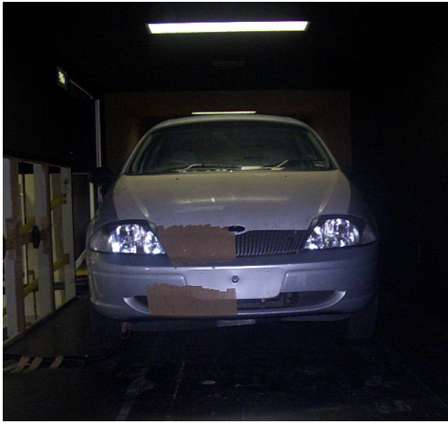
Figure 3: Side-to-side method (1/2 cooling air intake area shielded).
