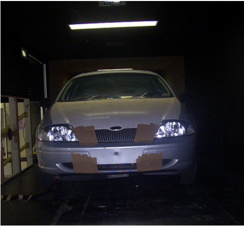
Figure 4: Side-to-centre method (1/2 cooling air intake area shielded).
