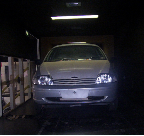
Figure 2: Horizontal method (1/2 cooling air intake area shielded).
