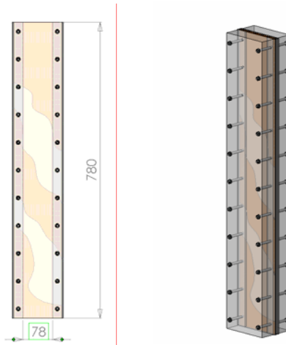
Figure 3 – Front and isometric view of the flat plate fuel-assembly-model, dimensions are in millimetres.
