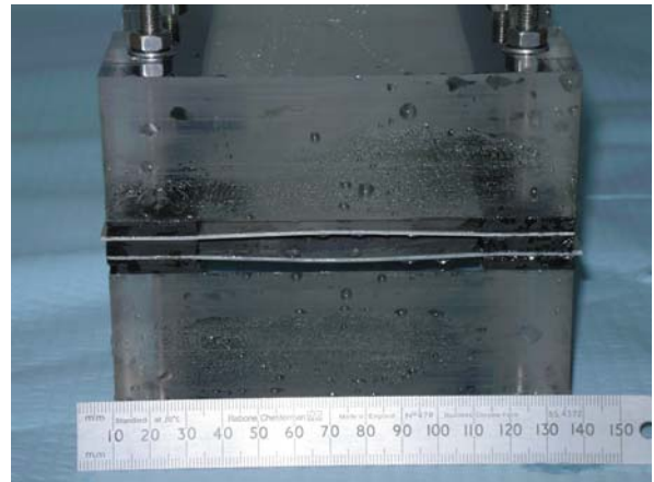
Figure 8 – Post-failure end view of the flat plate fuel-assembly-model. Note: both plates’ leading edges have buckled and plastically deformed away from each other.
