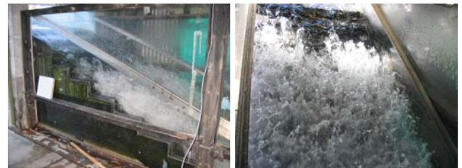
Figure 1. Skimming flow down a stepped chute (h = 0.1 m) (Configuration 3 d_c/h = 1.3 , Re = 7.3 E+5 ). Left: side view. Right: Top view with flow from top to bottom.
