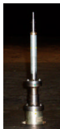
Figure 3: Motorised Ball Supporting Device mounted on a 6-Component Force Balance
