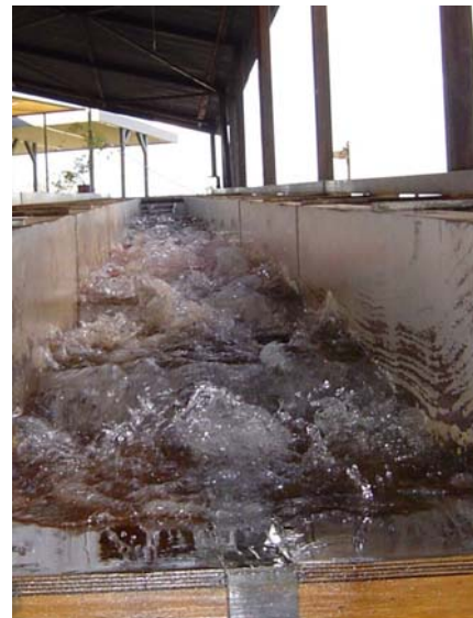
(B) Present study: Q(t=0+) = 0.065 m 3 /s, step 16, looking at advancing surge (Courtesy of C.G. SIM and C.C. TAN) Fig. 1 - Photographs of dam break and resulting surging wave.
