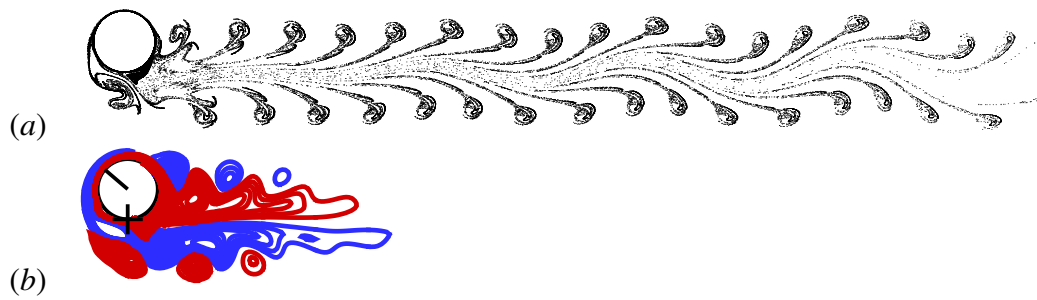
Figure 8.12: Flow produced by a cylinder free in the horizontal axis with a velocity ratio V_r = 1.25 between the translational and rotational oscillatory motions. Shown are: (a) fluid particle transport from ten massless particle sources placed near the cylinder surface, and (b) instantaneous vorticity contours. The cylinder is shown at its maximum vertical position and with its maximum anti-clockwise rotation.
