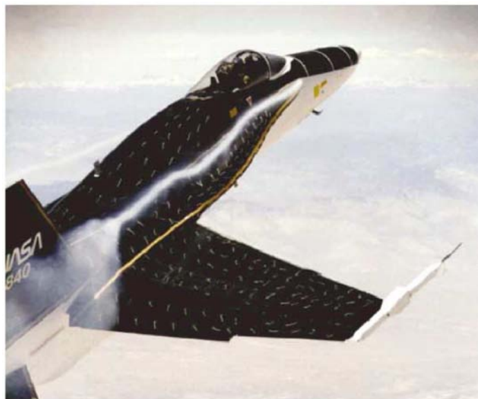
Figure 1.1: Smoke visualisation of a leading strake vortex from a military jet (FA-18). Vortex breakdown is seen here towards the tail fin of the aircraft as a bursting of the vortex (Mitchell & Delery 2001).
