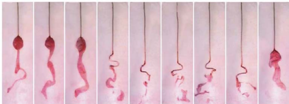
Figure 2.6: The transition in a pipe of the bubble breakdown to spiral breakdown, under the influence of an m = 1 excitation by Kurosaka et al. (2003). Flow is from the top of the image to the bottom, with time series incrementing from left to right.
