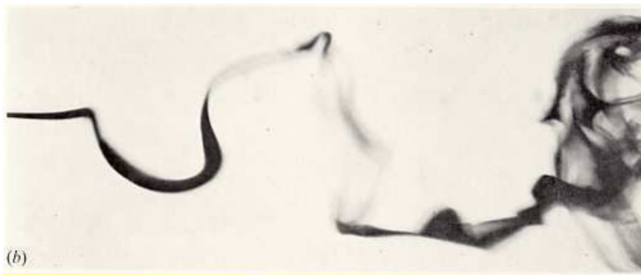
Figure 2.5: Spiral form of breakdown, identified here in the pipe flow of Sarpkaya (1971).
