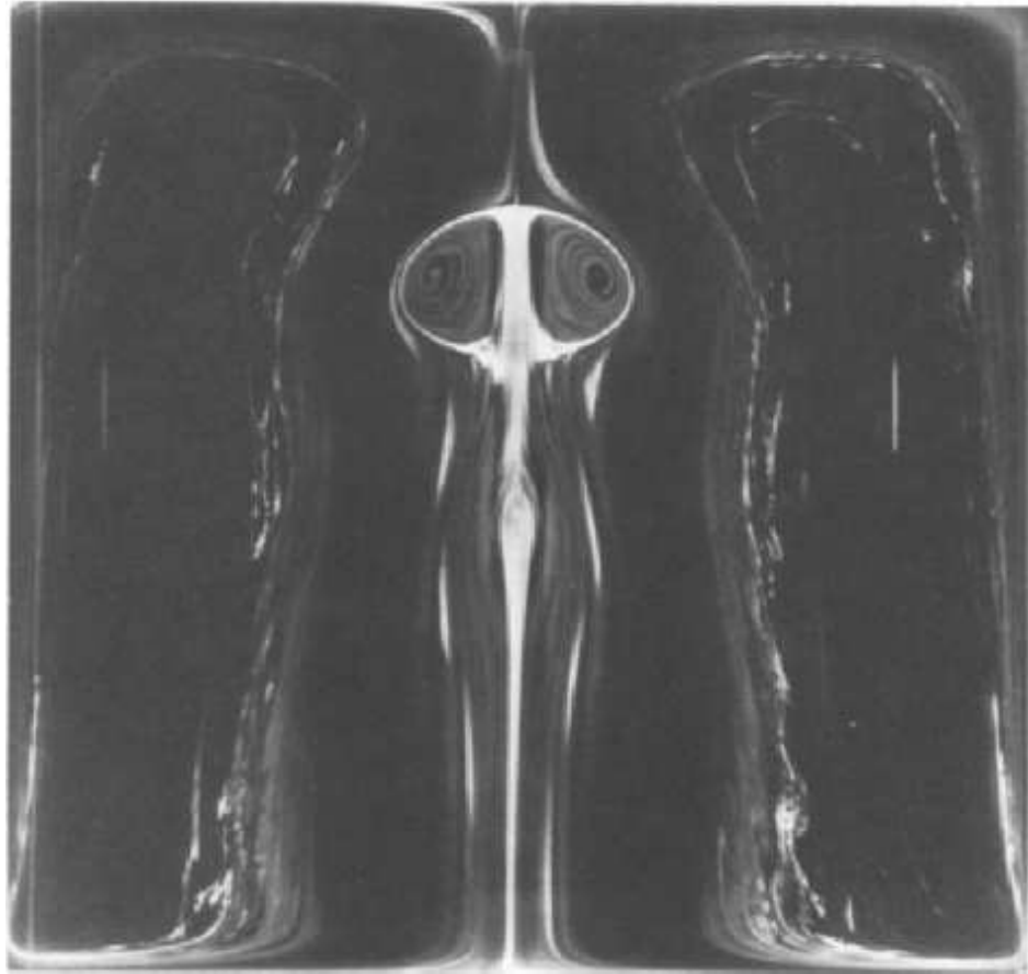
Figure 2.2: The vortex breakdown formed inside a closed cylinder. Shown here is an experimental result from the study of Escudier (1984) in a torsionally driven cylinder. The rotating base-plate is at the bottom of the image, and illumination of fluorescein dye is in meridional plane through the central axis.
